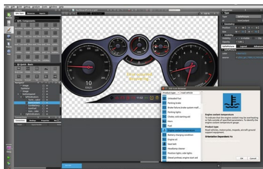
Figure 5. ISO icons added in Qt Quick Designer for use by Qt Safe Renderer
